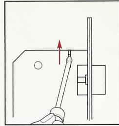
Insert screwdriver into top notch on lock and push up.
